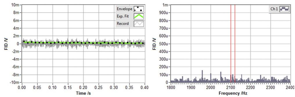
Figure 4a: Result of a "conventional" SNMR measurement for pulse moment  $Q$  of 12 Ams. Shown is the 16 times averaged FID voltage signal of the 72-turn Rx loop after a 30,000 times amplification. All loops (Tx, Rx, PP) have a diameter of 2 m. Noise cancelation with Remote Reference Technique. Location: Linum near Berlin.
