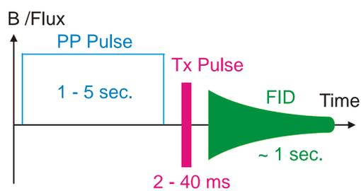
Figure 2: New SNMR Pulse sequence: Pre-Polarization Pulse before Tx excitation Pulse and FID recording.
