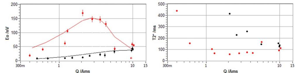
Figure 5: SNMR sounding without (black dots) and with pre-polarization (red dots). Same parameter as in Figure 3. Left: Initial amplitude  $E_0$ , right: relaxation time  $T_2^*$ . Location: Linum
