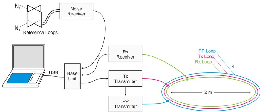
Figure 1: Schema of our SNMR instrument MRS-MIDI-III with pre-polarization.
