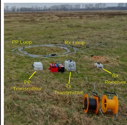
Figure 3: SNMR measuring system MRS-MIDI-III with pre-polarization during a field test.
