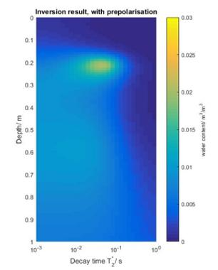
Figure 6: 1-D Q-T inversion result for data with pre-polarization.
