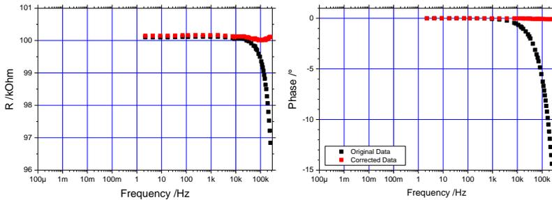
Impedance measurement on a 100 kΩ resistor. Black dots: Original data, red dots: Corrected data.
