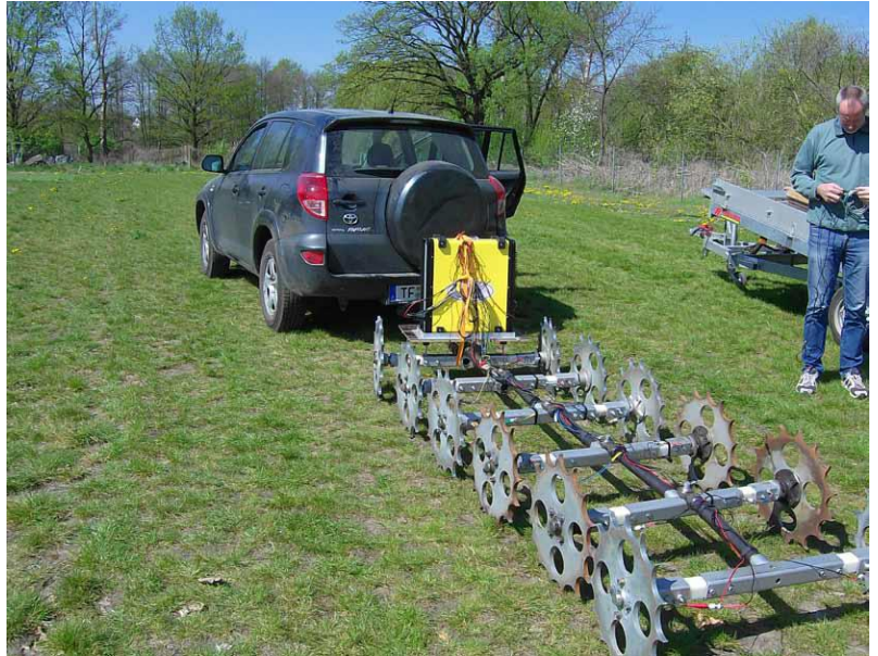
Fig. 1: SIP Rabbit during field operation. Yellow casing: Rabbit instrument.
