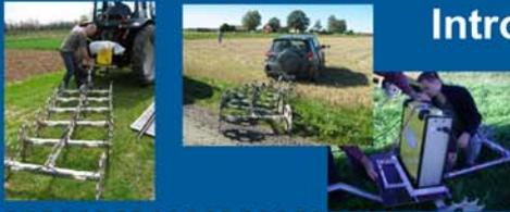
Geophilus electricus was developed to measure continuously the apparent electrical conductivity (ECa) at five depth intervals. It allows the delineation of conductivity structures in the three spatial dimensions and the transformation of the measured structures in a subsurface model.
